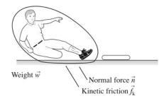
**Solve:** There are three forces acting *on* the baseball player due to his interactions with the two agents earth and ground. One of the forces *on* the player is the long-range weight force *by* the earth. Another force is the normal force exerted *by* the ground due to the contact between him and the ground. The third force is the kinetic friction force *by* the ground due to his sliding motion on the ground.
