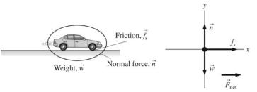
There are contact forces where the car touches the road. One of them is the normal force of the road on the car. The other is the force of static friction between the car's tires and the road, since the car is accelerating from a stop. The only long-range force acting is the weight of the car. Compare to Figure 4.31 and the discussion of propulsion in the text.
