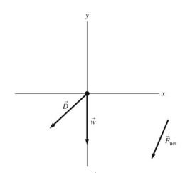
The acceleration (not shown) is in the same direction as  $\vec{F}_{net}$ . The velocity (not shown) is up to the right, opposite the drag force.
