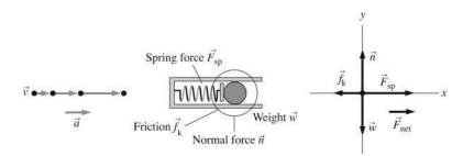
**Solve:** A force-identification diagram, a motion diagram, and a free-body diagram are shown. **Assess:** Since the normal force acting on the ball and the weight of the ball are equal in magnitude and opposite in direction, the ball experiences no vertical motion. Since the spring exerts a greater force on the ball than kinetic friction, the ball accelerates out the barrel of the gun.
