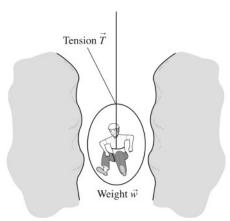
**Solve:** There are two forces acting on the mountain climber due to her interactions with the two agents earth and rope. One of the forces *on* the climber is the long-range weight force *by* the earth. The other force is the tension force exerted *by* the rope.
