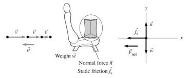
**Solve:** A force-identification diagram, a motion diagram, and a free-body diagram are shown. **Assess:** Since the normal force acting on the bag of groceries and the weight of the groceries are equal in magnitude and opposite in direction, the bag experiences no vertical motion. The only horizontal force acting on the bag of groceries is static friction, and it provides the net force acting on the bag which results in the acceleration of the bag.
