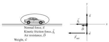
Assess:  $F_{net}$  points to the left, as does the  $\vec{a}$  for a car that is moving to the right but slowing down.
