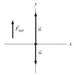
(b) Since the froghopper is accelerating upward the net force is upward; hence, the upward force of the ground on the froghopper is greater than the downward gravitational force (the froghopper's weight).
