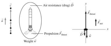
**Solve:** A force-identification diagram, a motion diagram, and a free-body diagram are shown. **Assess:** You now have three important tools in your "Physics Toolbox," motion diagrams, force diagrams, and free-body diagrams. Careful use of these tools will give you an excellent conceptual understanding of a situation.
