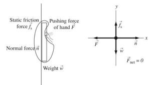
Assess: The net force is zero, as it should be for an object which is motionless (isn't accelerating).
