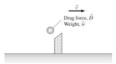
The environment touches the ball at the ball's surface. The force on the ball's surface is the drag force, and this is the only contact force on the system. The drag force is always opposite to the direction of motion of an object. The only long-range force acting is the ball's weight.
