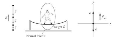
**Solve:** A force-identification diagram, a motion diagram, and a free-body diagram are shown. **Assess:** There are only two forces on the gymnast. The weight force is directed downward and the normal force is directed upward. Since the gymnast is slowing down right after after making contact with the trampoline, upward normal force must be larger than the downward weight force.
