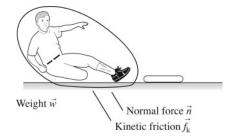
**Solve:** A possible description is, "A baseball player is sliding into second base." Assess: On the free-body diagram, kinetic friction force is the only horizontal force, and it is pointing to the left. This tells us that the baseball player is sliding to the right.
