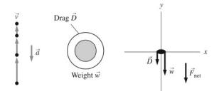
**Solve:** A force-identification diagram, a motion diagram, and a free-body diagram are shown. **Assess:** The drag force due to the air is opposite the motion.
