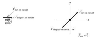
The magnet's mounting is what provides the force that keeps the magnet in place. The force of the magnet on the mount is equal and opposite to the force of the mount on the magnet, since these are action/reaction pairs. Using Newton's third law,
