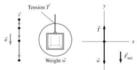
**Solve:** A force-identification diagram, a motion diagram, and a free-body diagram are shown. **Assess:** You now have three important tools in your "Physics Toolbox," motion diagrams, force diagrams, and free-body diagrams. Careful use of these tools will give you an excellent conceptual understanding of a situation.
