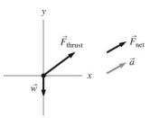
**Solve:** (a)–(c) There is a thrust at an angle to the horizontal and a weight. There is no normal force so the object is not on a surface. Adding the thrust and the weight we obtain a net force that acts as shown in the figure. The acceleration acts in the direction of the net force.
