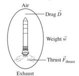
**Solve:** A possible description is, "A rocket accelerates upward." **Assess:** It is given that the net force is pointing up. Then,  $\vec{F}_{net} = \vec{F}_{thrust} - \vec{w} - \vec{D}$  must be greater than zero. In other words,  $\vec{F}_{thrust}$  must be larger than  $(\vec{w} + \vec{D})$ .
