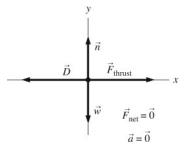
Solve: (a)–(c) Since the net force is zero, the acceleration will also be zero.
