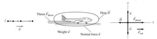
**Solve:** A force-identification diagram, a motion diagram, and a free-body diagram are shown. **Assess:** You now have three important tools in your "Physics Toolbox," motion diagrams, force diagrams, and free-body diagrams. Careful use of these tools will give you an excellent conceptual understanding of a situation.
