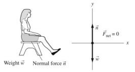
(a) The passenger is sitting on a *very* slippery bench in a car that is traveling to the right. Both the passenger and the seat are moving with a constant speed. There is a force on the passenger due to her weight, which is directed down. There is a contact force (the normal force) between the passenger and the seat, which is directed
