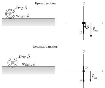
The only contact force is the force of air drag on the ball. The only long-range force is the weight of the ball. Drag always points in the direction opposite to the motion. From the free-body diagram, the net force will always be greater when the beach ball is moving upward compared to downward. There the weight of the ball and the drag force always reinforce each other.
