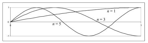
For a resonant condition, the free end of the string will be an antinode, and the fixed end of the string will be a node. The minimum distance from a node to an antinode is  $\lambda/4$ . Other wave patterns that fit
